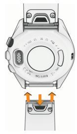
**NOTE:** Make sure the band is secure. The latch should close over the watch pin.
