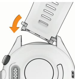
**NOTE:** Make sure the band is secure. The watch pin should align with the holes on the watch.
